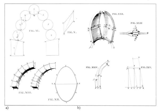
Fig. 5 Structural analysis of St.Peter's dome from Poleni's "Historical Records of the Great Dome of the Temple" - Vatican 1748: a) theory of the curve of thrust, b) application of the principle of virtual work
