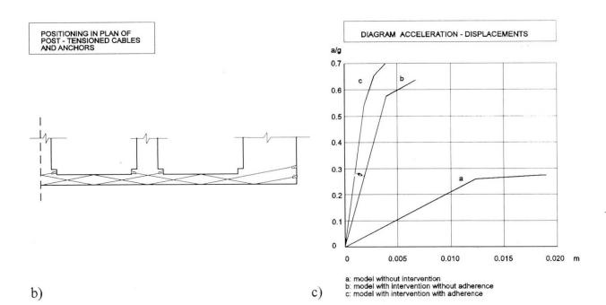
Fig. 15 Palazzo Altemps: prestressed cables to reinforce the remaining upper part of a demolished wall, working now as a "beam", to allow support for the floors above
