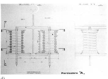
provisional steel elements connected to a monitoring system are going to be used to recover the huge deformations created by ancient soil settlements.
