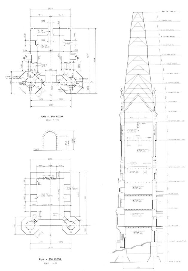
Fig. 1 Elevation and cross-sectional view of the tower.
