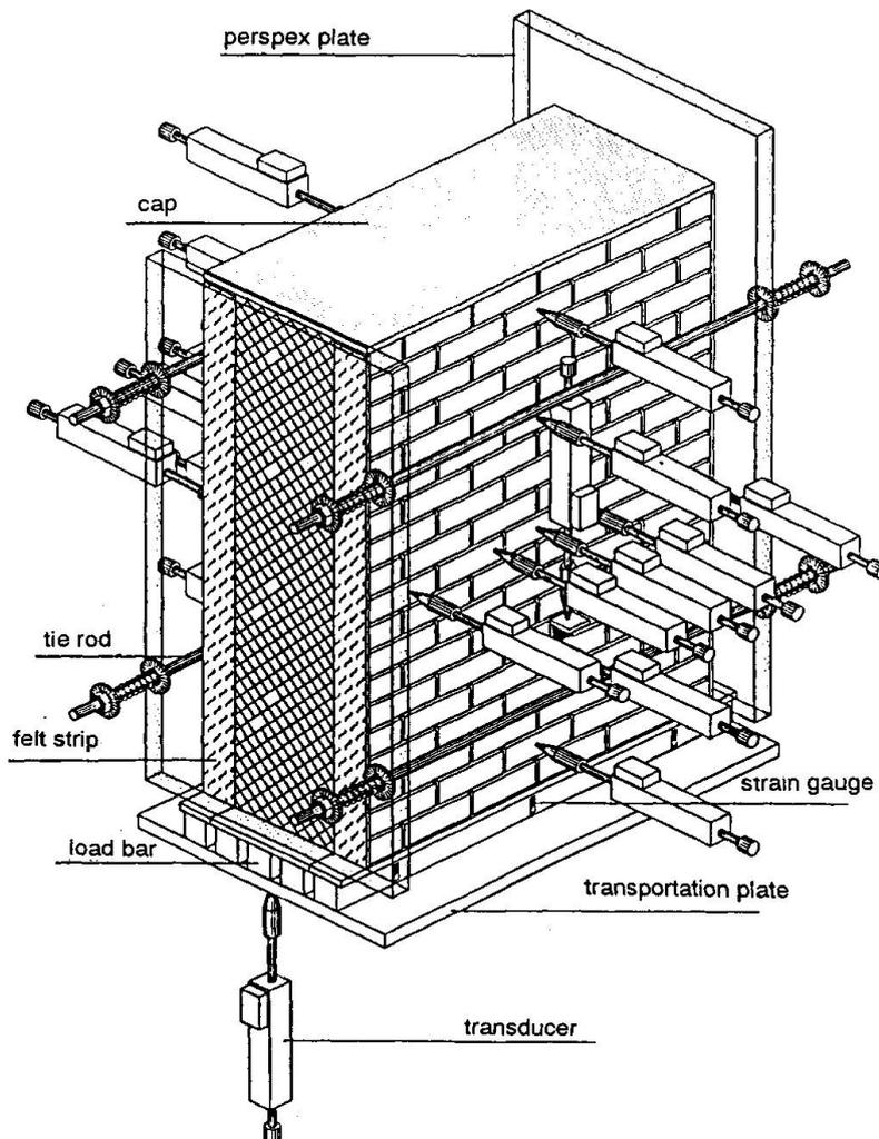
Fig. 2 specimen ( $t_i/t_a = 3$ ) with the measure equipment
