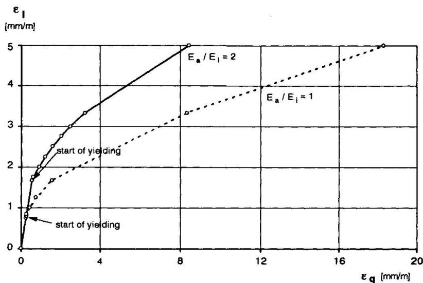
– In the case of a weaker infill the collapse of the system is caused by a compressive edge failure due to bending of the outer skins. Large bending deflections combined with gapping of the bed joints or bending cracks announce the failure long time before. The slenderness and the boundary conditions of the outer skins have an important influence of the load bearing capacity of multiple leaf masonry.
