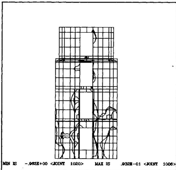
Fig. 5 STRESSES DUE TO SISMIC ACTIONS
