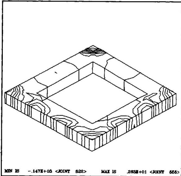
Fig. 7 STRESSES AT FIRST FLOOR LEVEL RIGID FOUNDATION
