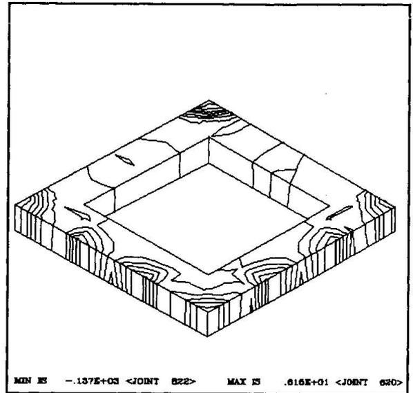
Fig. 8 STRESSES AT FIRST FLOOR LEVEL ELASTIC FOUNDATION
