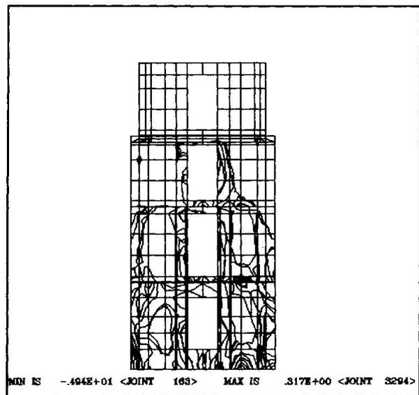
Fig. 6 STRESSES DUE TO SISMIC ACTIONS
