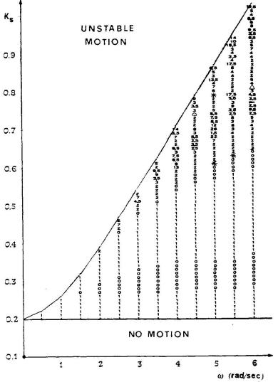
FIG. 10. Multiblock column: stable or unstable motions [5,7].
