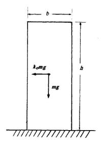
FIG. 1. Monolithic column.
