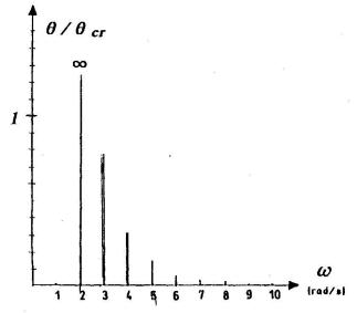
FIG.12. Typical distribution of max. rotation for the column of Fig. 10.
