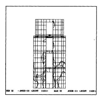
Fig. 5 STRESSES DUE TO SISMIC ACTIONS HOMOGENEOUS MATERIAL
