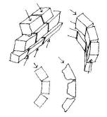
Fig.4 - Facing failure mechanisms
