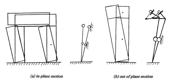
FIG. 9. One d.o.f. trilith mechanism.
