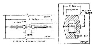
Fig.5 Drum's interface and shear key (After Penrose, C.K. (1973))
