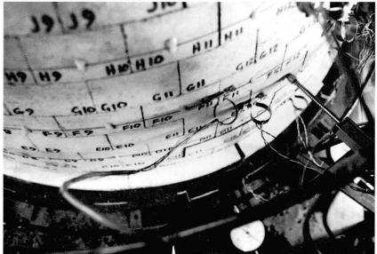
fig. 7 - Crack pattern for outward horizontal sliding of the base
