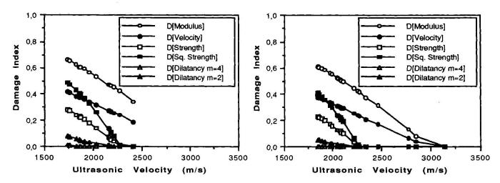
Fig. 5 & 6: Damage indices resulting from the various formulations for the damaged and restored column
