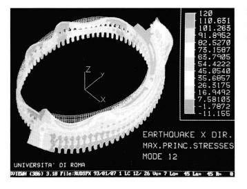
fig. 11 - Analytical model of the today configuration. Spectrum response dynamic analysis.
