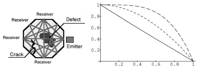
Fig. 1 : Multi path scanning for defect positioning
