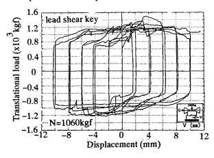
Fig.16 Behavior of interface with lead shear key under cyclic loading
