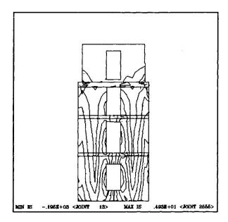
Fig 1 . STRESSES ON FACADES RIGID FOUNDATION
