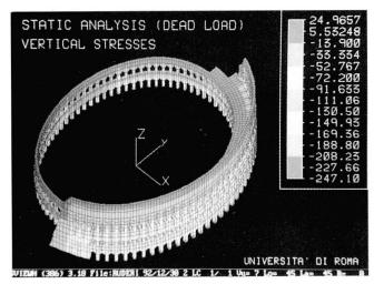
fig. 10 - Analytical model of the today configuration
