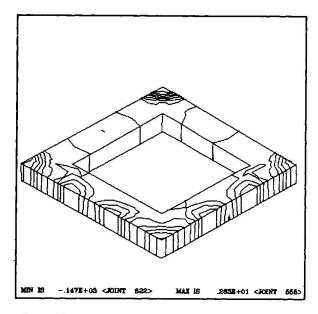
Fig. 7 STRESSES AT FIRST FLOOR LEVEL RIGID FOUNDATION
