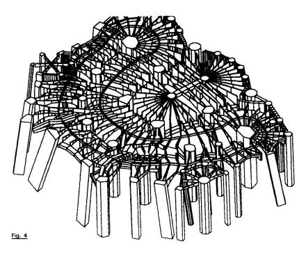
result was the computer model represented in Fig. 4 and some preliminary analyses were carried out to discover its performance. The lead joints on the central columns at their junction with the pedestal and the capital were treated alternatively as completely fixed or rotationally free hinges.
