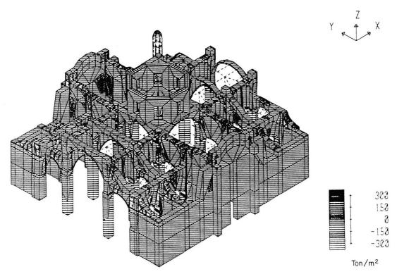
$\underline{\text{Fig. 6}}$  State of stress due to gravity loading from a finite element analysis of the central portion of the Cathedral
