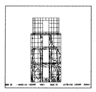
Fig. 6 STRESSES DUE TO SISMIC ACTIONS HETEROGENEOUS MATERIAL
