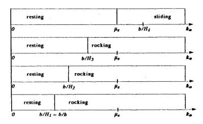
FIG. 8. Starting modes for multiblock column.
