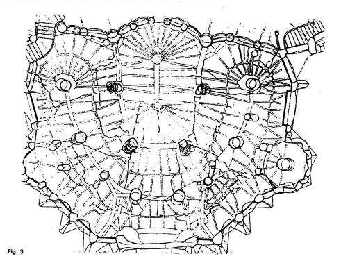
Detailed analysis through direct observation and an exhaustive photographic survey of over 1 000 images has enabled us to determine the pattern of cracks we reproduce here, which is only an overall view amongst all those that were detected. (Fig. 3)
