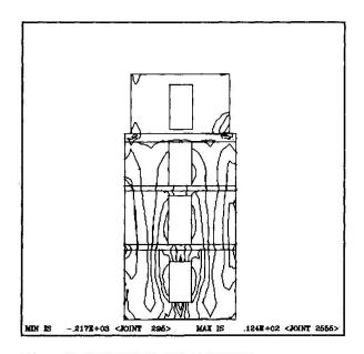
Fig. 2 STRESSES ON FACADES ELASTIC FOUNDATION
