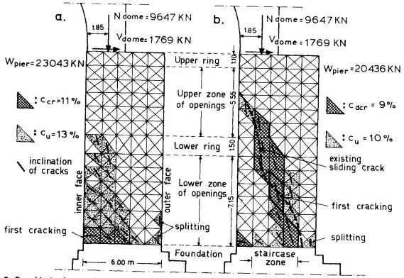
Fig.6 Predicted cracking patterns of the piers  $P_1$  and  $P_2$  till failure: a.Massive pier  $(P_1)$ , b.Pier with staircase  $(P_2)$
