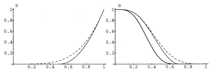
Fig. 3.a : Damage evolution as a function of stress level σ/f<sub>k</sub>, as predicted by dilatancy
