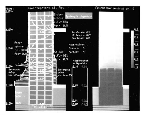
Fig. 8 Effect of an water repellent plaster
