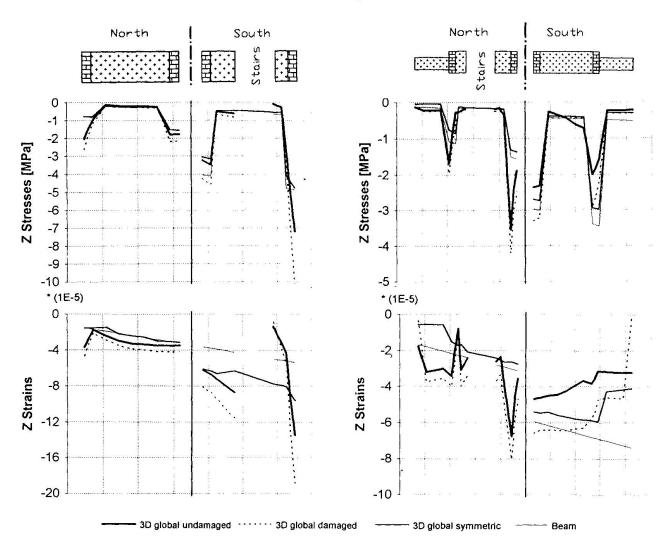
Fig. 10 - Stresses and strains at the first loggia: comparison among different models
