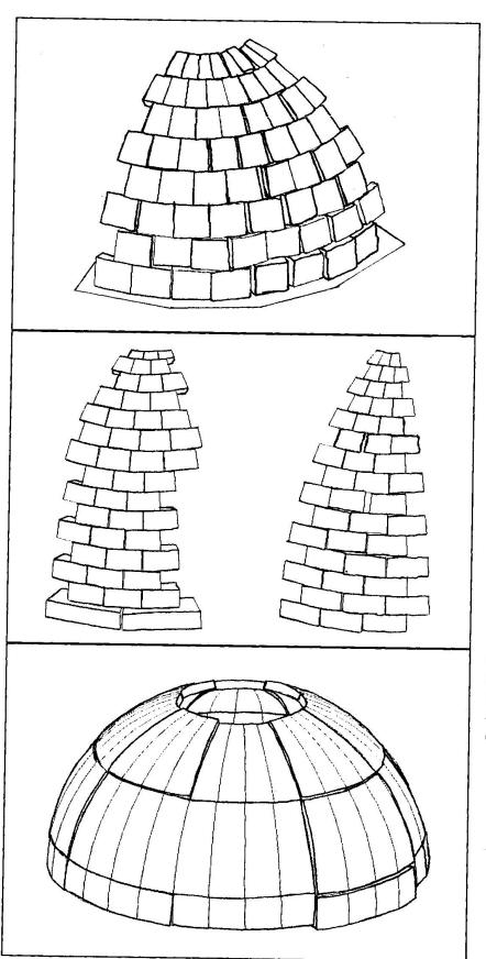
fig.2-A 90° sector of a spherical dome subjected to horizontal outward action on the second row
