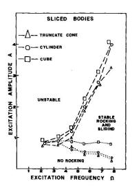
Fig 10. Summary of sinusoidal tests for sliced bodies
