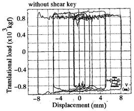
Fig.15 Behavior of interface without shear key under cyclic loading
