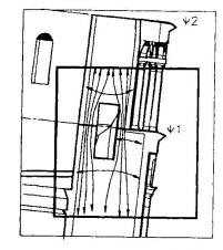
Fig.2 - Critical zone of the Tower at the first loggia
