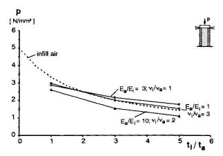
Fig. 5 FE-analysis: maximum of average applied stress (p) for reaching the critical edge stress at different thickness ratios  $(t_i/t_a)$
