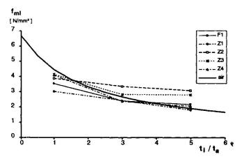
Fig. 6 Experiments: crushing strengths  $(f_{ml})$  of filled and unfilled specimens of different thickness ratios  $(t_i/t_a)$
