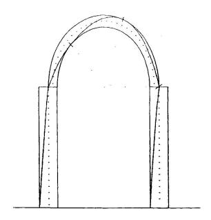
Fig. 9 The thrust line tracing to verify the results obtained by the kinematical procedure
