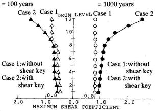
Fig.10 Results of non-linear response analysis; Distribution of the maximum shear coefficient along height of a column without beam and pediment on its capital
