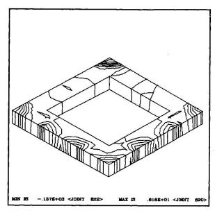
Fig. 8 STRESSES AT FIRST FLOOR LEVEL ELASTIC FOUNDATION
