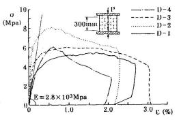
Fig.6 Stress – strain relationships from compressive tests
