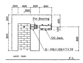
Fig.1 In-plane flexural test
