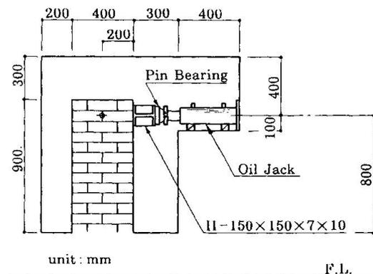
Fig.1 In-plane flexural test
