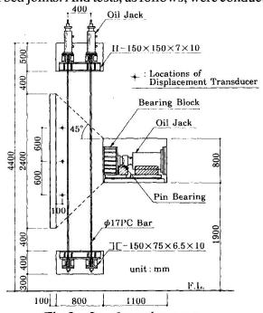
Fig.2 In-plane shear test
