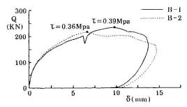
Fig. 4 Load – displacement relationships for In–plane shear test
