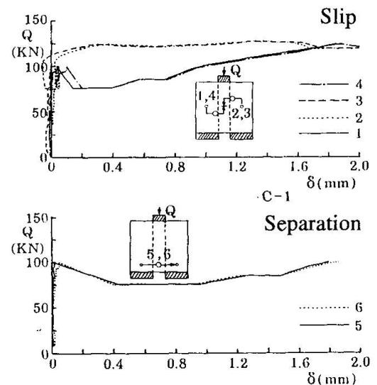
Fig.5 Load – displacement relationships at the joints
