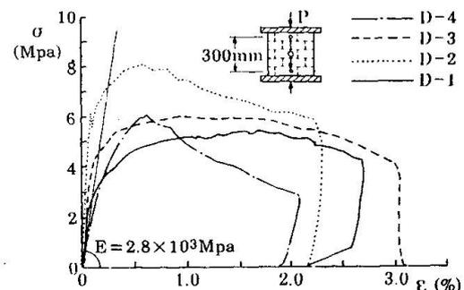
Fig.6 Stress – strain relationships from compressive tests
