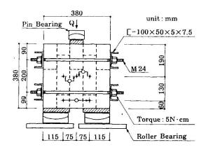
Fig.3 Double shear test
