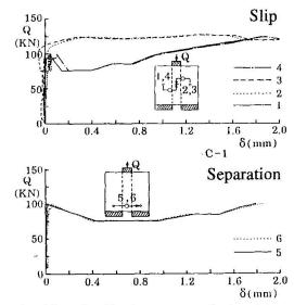
Fig. 5 Load – displacement relationships at the joints
