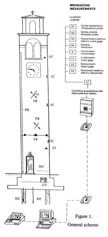
All the difficulties encountered in the steps for detection and diagnostic can obtain a powerful aid by monitoring the main parameters of the structure with non destructive techniques.
