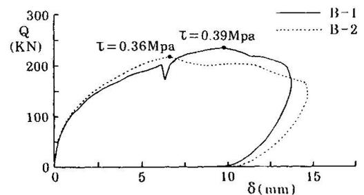
Fig.4 Load – displacement relationships for In-plane shear test
