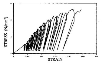
Fig. 2 - Stress-strain curve of strain gauge 7 - specimen 2.
