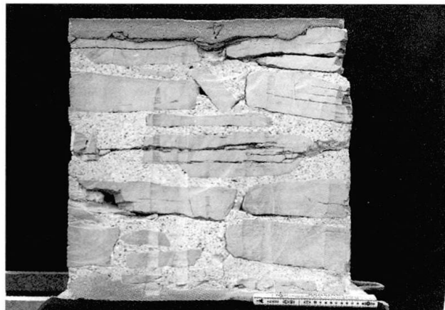
Photo 6 - Sample obtained from inner masonry.
