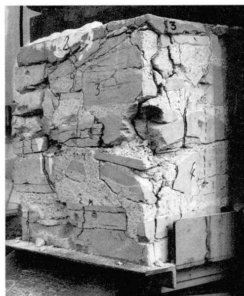
Photo 7 - Collapse of specimen No. 3.
