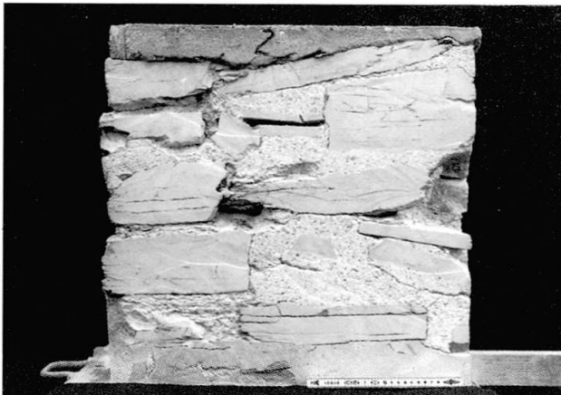
Photo 5 - Sample obtained from inner masonry.
