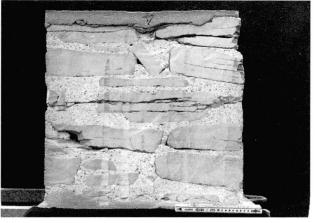
Photo 6 - Sample obtained from inner masonry.
