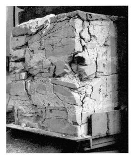
Photo 7 - Collapse of specimen No. 3.
