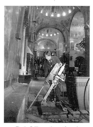
Fig. 3 - Drilling equipment for coring the foundation masonry
