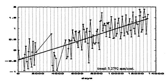
Figure 3: O.D. data (years 1956-1992), base no. 5: linear regression (values in mm [positive values=cracks opening])
