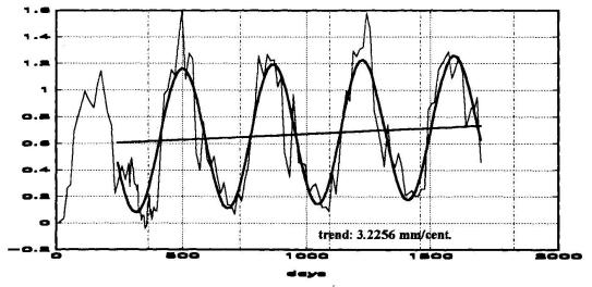
Figure 5: trend analysis of S.B.A.A. data (years 1956-1992), deformeter no. 6, web no. 4: linear plus harmonic approximation (values in mm [positive values=cracks opening])
