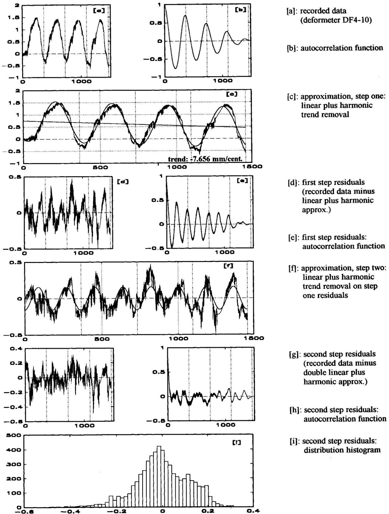
Figure 2: Trend removal procedure; application on data recorded by deformer no. DF4-10 (web no. 4, internal dome, lower part [negative values=cracks opening])
