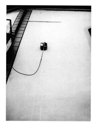
Fig. 2: The 500 MHz-antennas in the reflection arrangement
