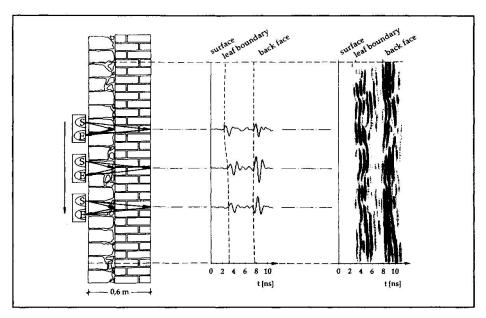
Fig. 3: The reflection arrangement on a multiple leaf wall; schematic cross section, received signals and radargram (S..transmitter, E..receiver, \( \psi\).. direction of profiling)
