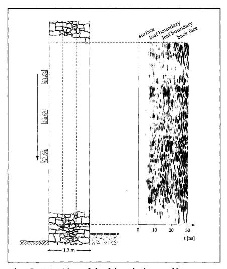
Fig. 7: Detection of leaf boundaries; wall cross
