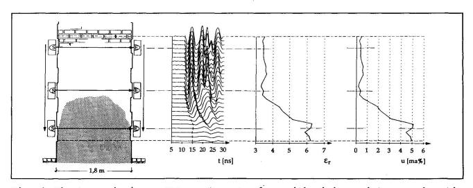
Fig. 4: The transmission arrangement on a column with rising moisture; schematic cross section, received signals, relative permittivity and moisture profile (S..transmitter, E..receiver, \dots.direction of profiling)
