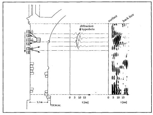
Fig. 9: The detection of anomalies with the reflection arrangement; wall cross section of the Matthiaskapelle in Kobern/Mosel, receiver signal and radargram
