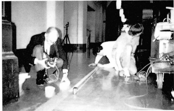
Fig. 10 Magnetic Detection & SASW Equipment
