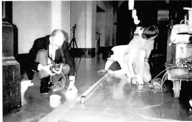
Fig. 10 Magnetic Detection & SASW Equipment
