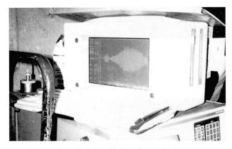
Fig. 8 Pulse Velocity Data on Field Computer
