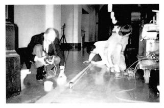
Fig. 10 Magnetic Detection & SASW Equipment
