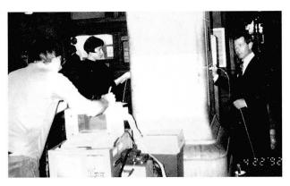
Fig. 7 Pulse Velocity Equipment in Use
