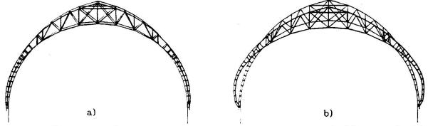
a) the deformed shape in the case of linear elastic analysis (Tr=700)
