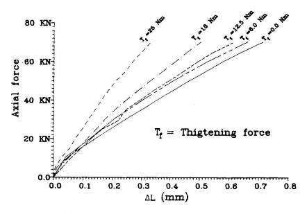
Fig.10 P-ΔL experimental behaviour for different tightening force
