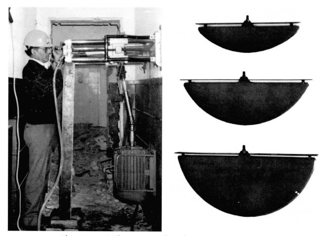
Fig. 3: Cutting operation in a flat jack test
