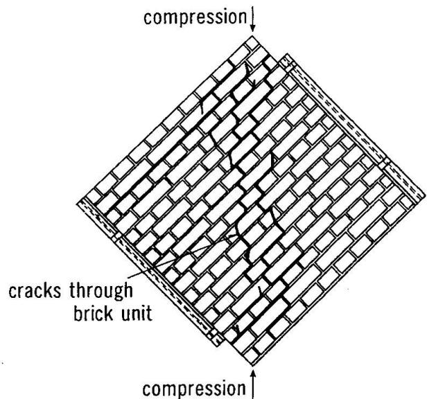
Fig. 11 Crack pattern of a retrofitted wall specimen
