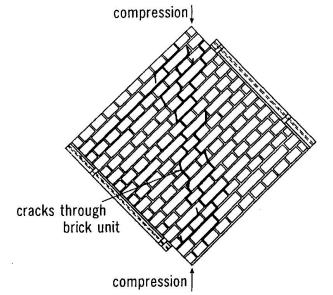
Fig. 11 Crack pattern of
