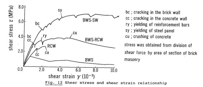
The retrofitted prototype was a brick masonry wall reinforced with steel elements, like Specimen BWS.
