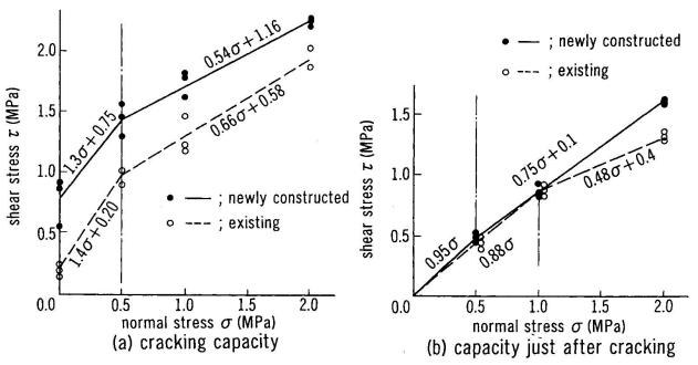
Fig. 8 Sliding shear capacities
