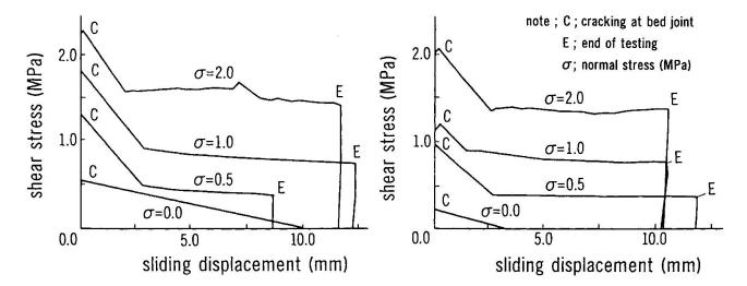
Fig.7 Shear stress and sliding displacement relationship
