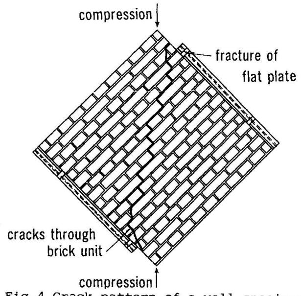
Fig.4 Crack pattern of a wall specimen
