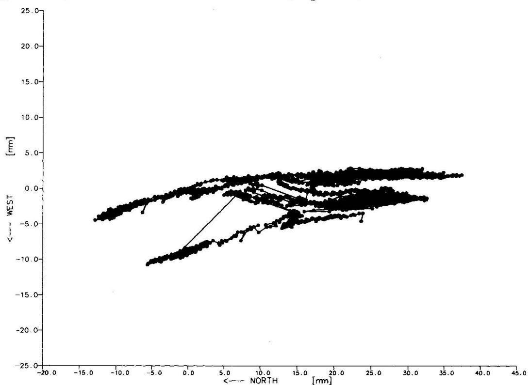
Figure 4: Planimetric displacements of the Cathedral dome
