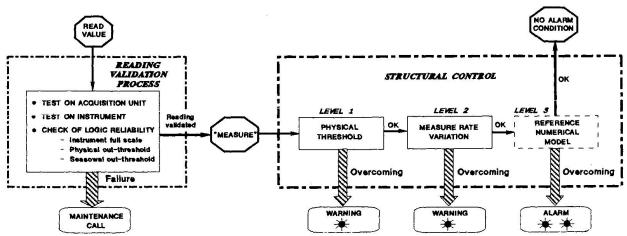
Figure 2: On line control architecture
