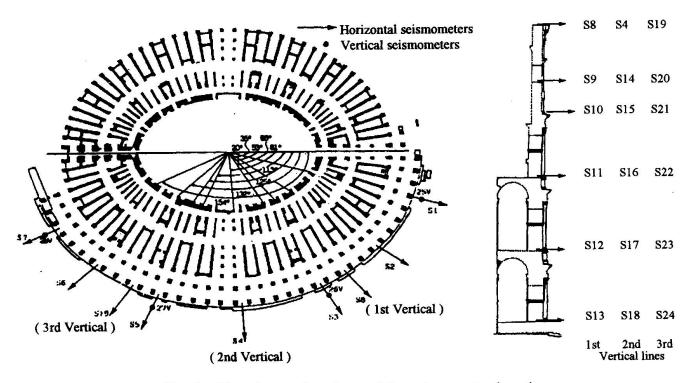
Fig. 1 Plan view and sections of the seismometer locations
