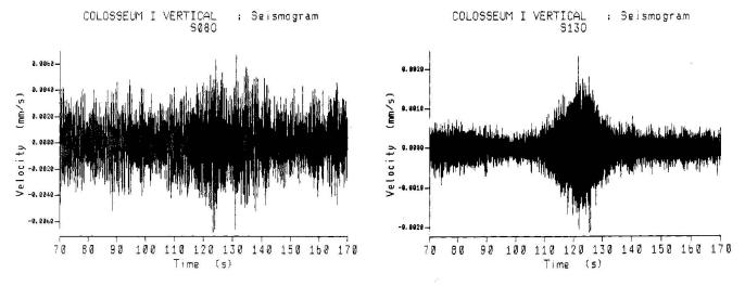
Fig. 2 Seismograms at locations S13 and S8 obtained during the transit of the train of the underground
