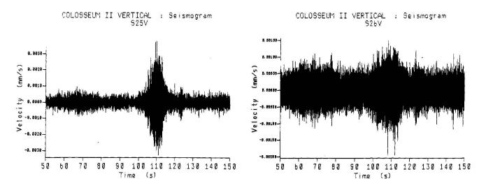
Fig. 7 Seismograms at locations 25V and 26V obtained during the transit of the train of the underground
