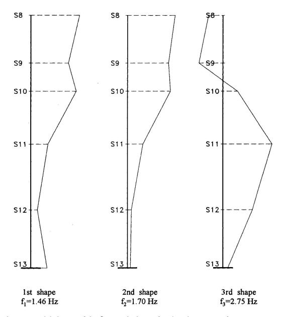
Fig. 3 Modal shapes of the first vertical associated to the structural resonances
