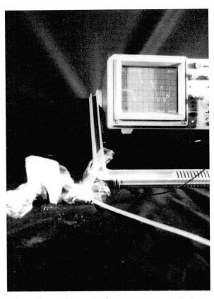
Fig. 8: Ultrasonic measurement to determine the mechanic properties of mortar
