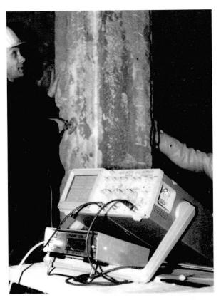
Fig. 7: Investigation of a sandstone pilar with the ultrasonic method
