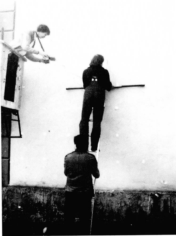
Fig. 3: Investigation with the geoelectric method
