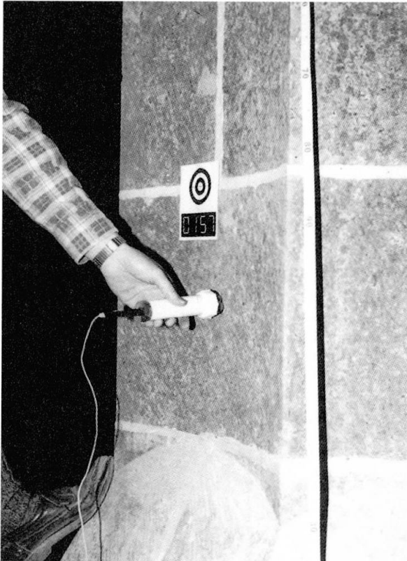
Fig. 5: Investigation with the self-potential method
