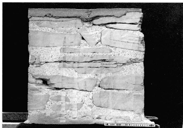
Photo 6 - Sample obtained from inner masonry.
