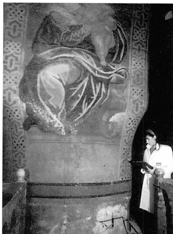
Fig. 7 - Measurement of the state of stress in a pillar by means of the flat-jack technique
