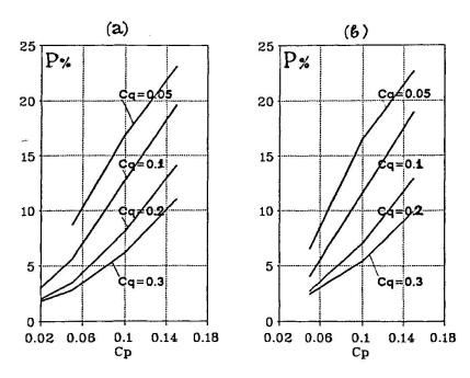
Fig. 3: Crack appearance probabilities in 6m-span slabs (a) and in 9m span slabs (b) vs. variation coefficient of presstress  $(C_p)$  for different variations of live load.
