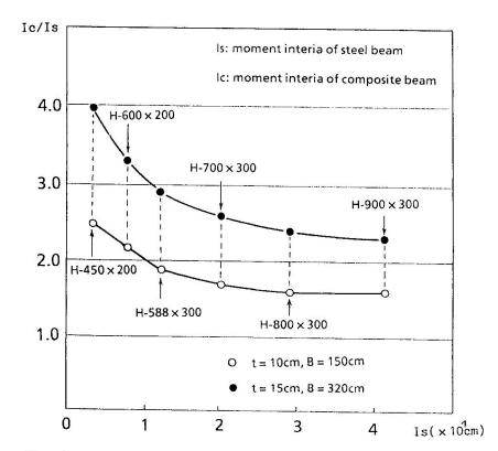
Fig.2 Increase in flectial rigidity of composite beam
