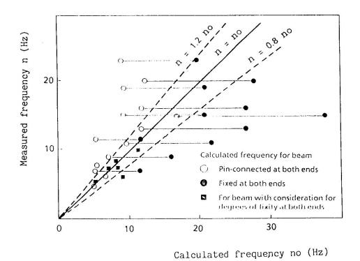
Fig.4 Frequency of floor beam
