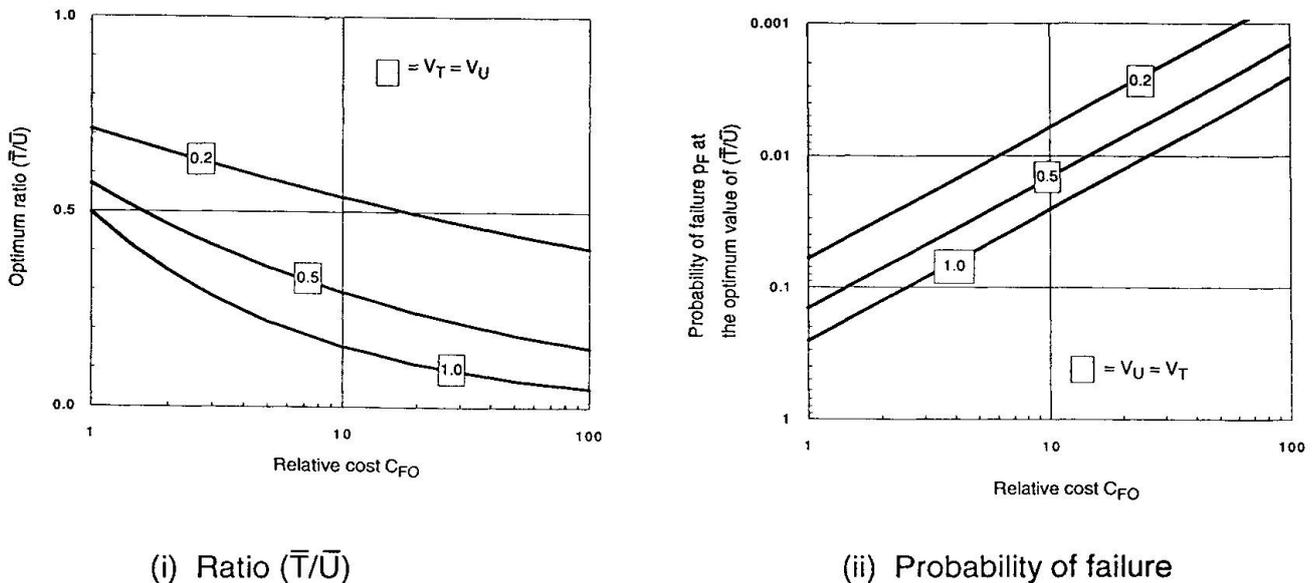
Fig. 2 Optimum values for design codes ( $m = 0.5$ ).
