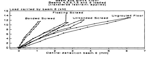
Figure 2: Influence of screed type on beam stiffness. (Transverse restraint applied)
