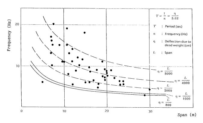
Fig.3 Measurement frequency VS. span
