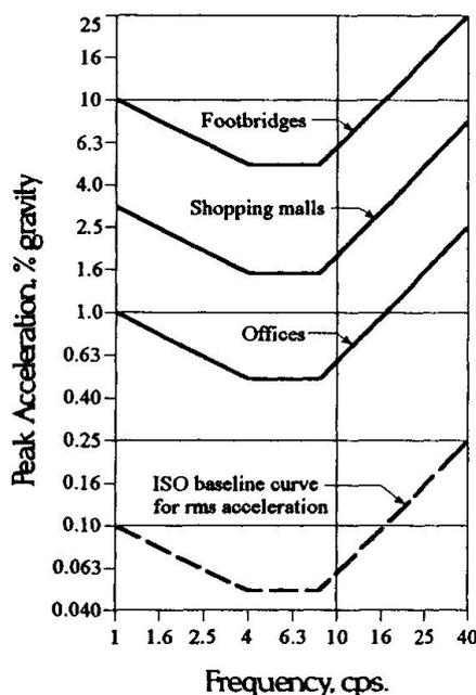
**Figure 1** Proposed Acceleration Limits for Walking Vibrations
