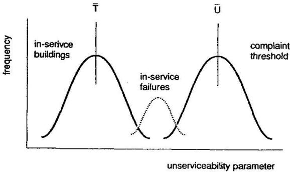
Fig. 1 Statistical model for a design code.
