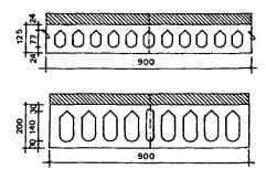
Fig. 2: Sections of analysed floor slabs.
