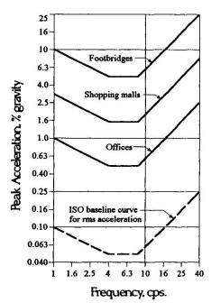
Figure 1 Proposed Acceleration Limits for Walking Vibrations
