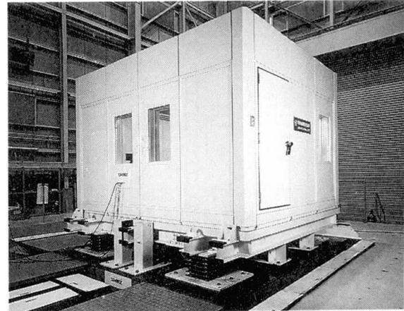
Fig.2 Vibration Simulator
