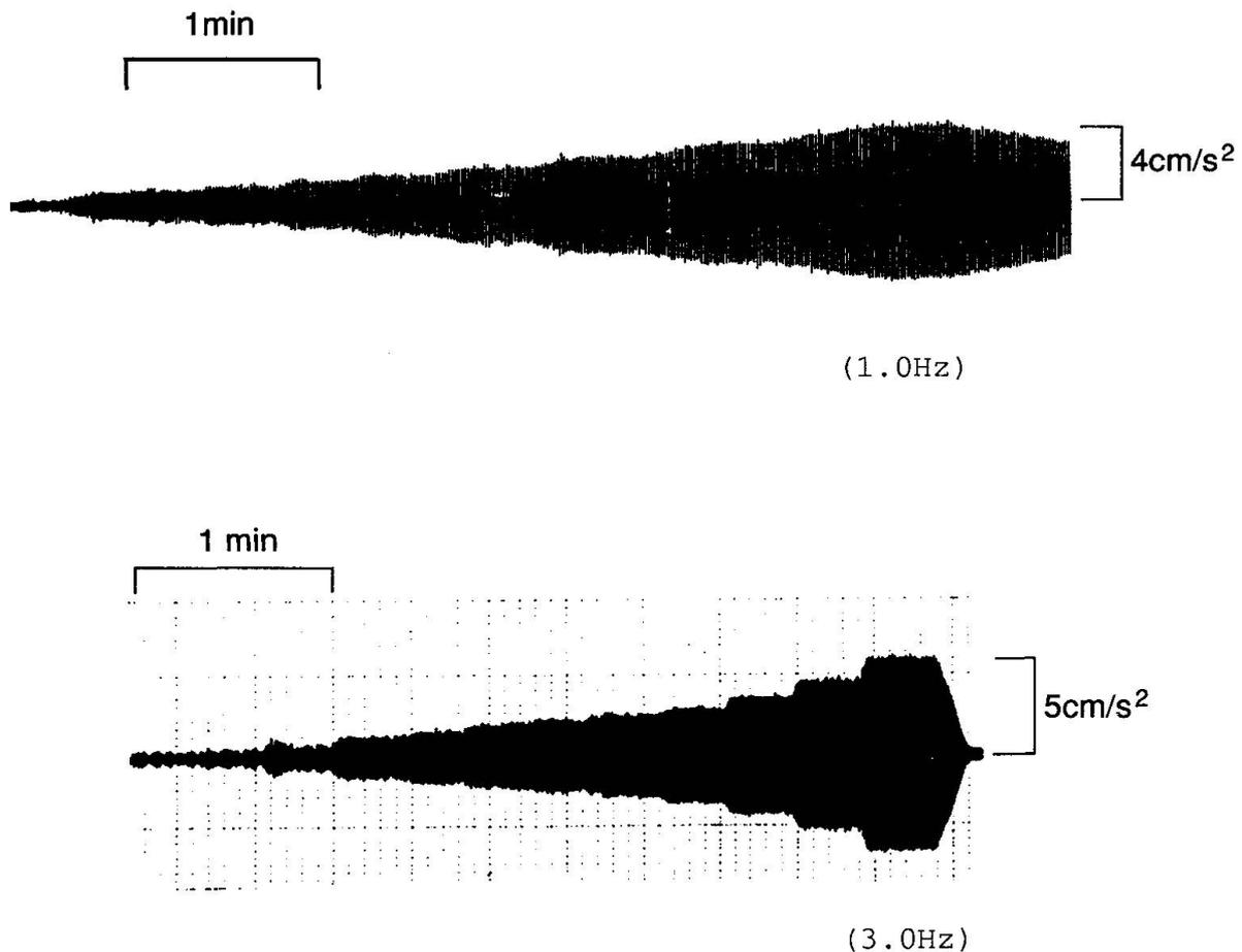
Fig.2 Examples of test room acceleration
