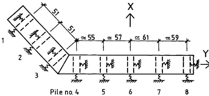
Compared to a structure on dry land, the submerged structure is – from the point of view of dynamic response – encumbered by enormous added masses related to vertical and horizontal movements as well as to water contained in the caissons and the chambers for absorption of wave energy.
