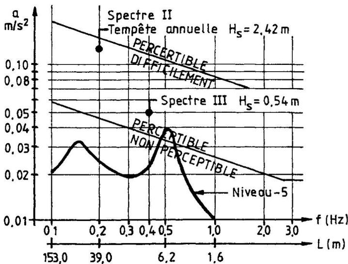
Fig. 7 Maximum acceleration for regular waves and for spectra II and III
