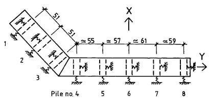
Compared to a structure on dry land, the submerged structure is – from the point of view of dynamic response – encumbered by enormous added masses related to vertical and horizontal movements as well as to water contained in the caissons and the chambers for absorption of wave energy.
