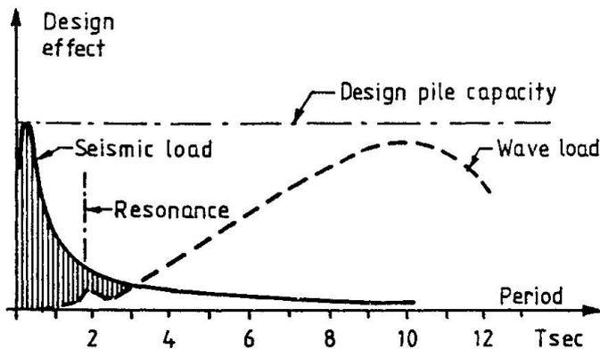
Fig. 6 Design effect on a piled foundation. (Alt. 3).
