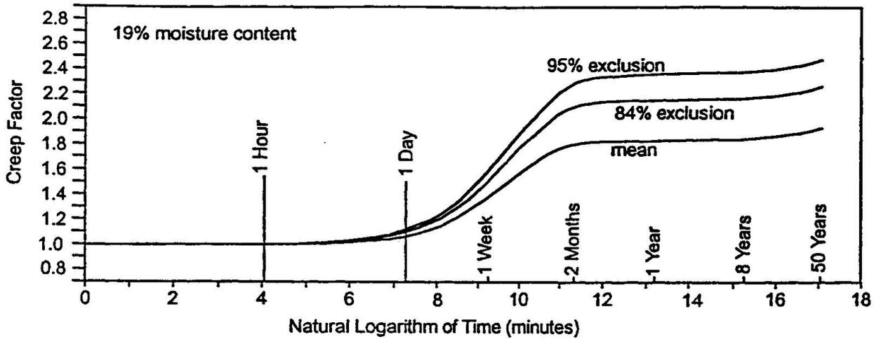
Fig. 1. Relative Creep Response of Structural Lumber [5].
