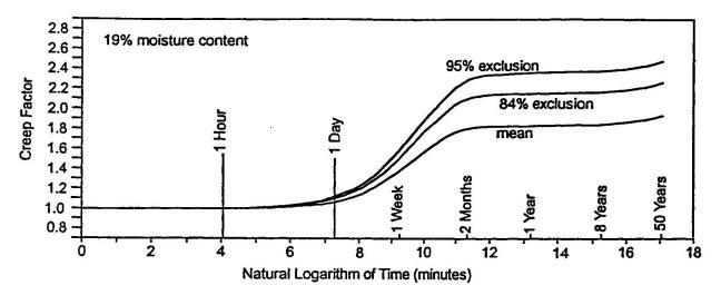
Fig. 1. Relative Creep Response of Structural Lumber [5].
