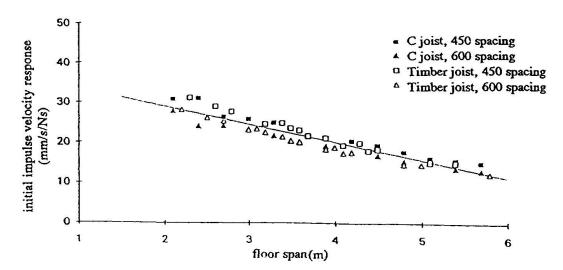
Fig.4 Impulse velocity response of Australian floors vs floor span (with floor mass plus 30kg/mm<sup>2</sup> live load)
