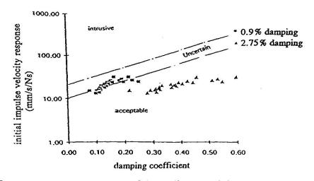
Fig.2 Impulse velocity response of Australian steel joist floors vs damping
