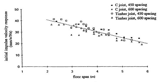
Fig.3 Impulse velocity response of Australian floors vs floor span (with floor mass only)
