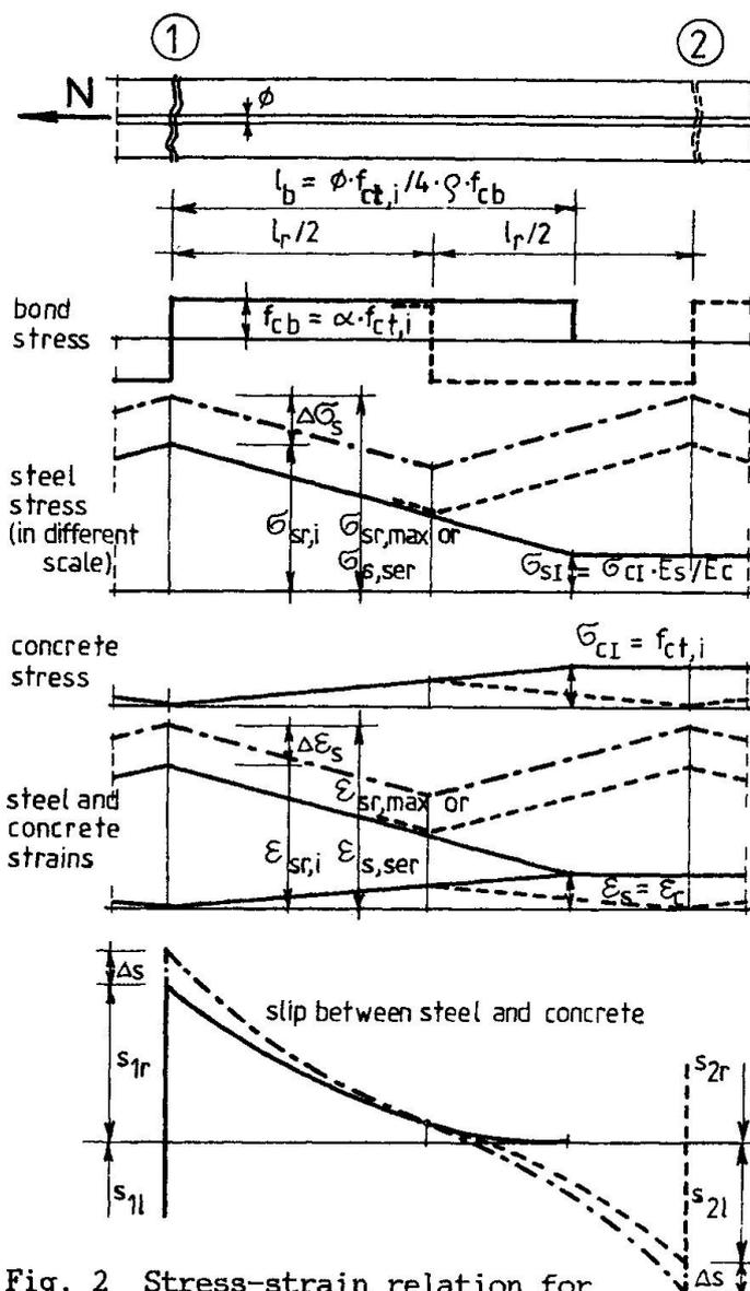
Fig. 2 Stress-strain relation for the calculation of crack width
