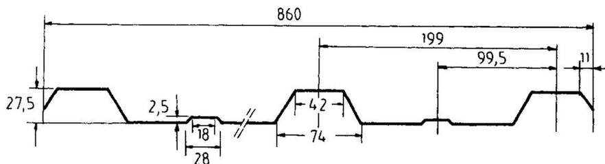
Fig. 1 Typical cross-section of the steel sheeting
