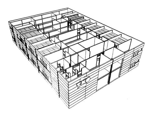
FIGURE 1: Isometrique view of non-structural components for building #11.
