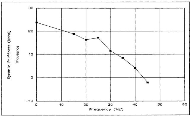
Figure 2: Stiffness vs Frequency Measurements for Prestressed Slab 1
