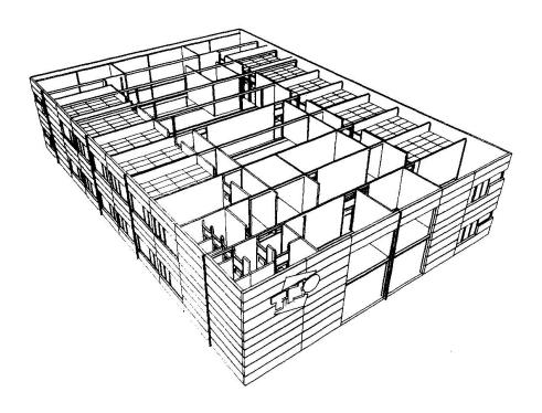
FIGURE 1: Isometrique view of non-structural components for building #11.
