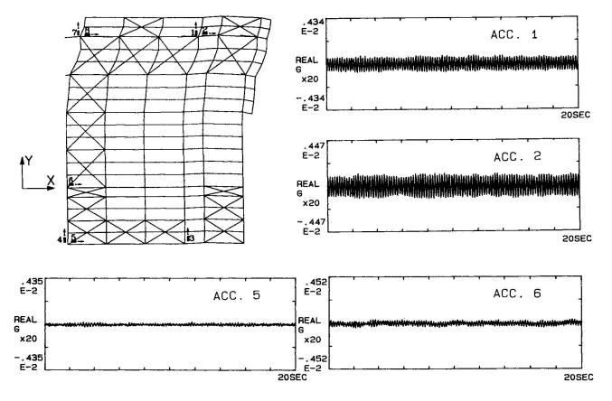
Fig. 5 - Mode 2 of the numerical model (5.95 Hz) and recorded accelerations at 5.5 Hz.
