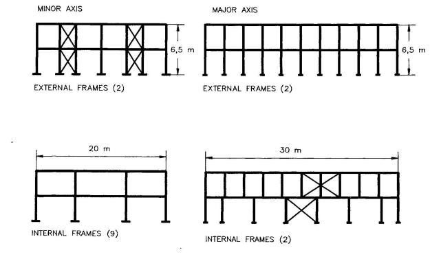
FIGURE 2: Schematic drawings of structrual frames for building # 11.
