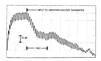
FIGURE 5: DECAY OF FLOOR VIBRATION (7.5 HZ)
