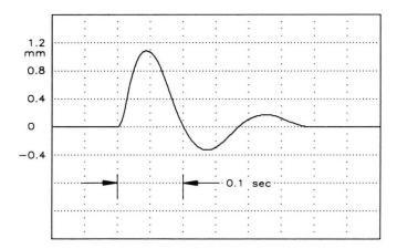
FIGURE 4: FLOOR DISPLACEMENT
