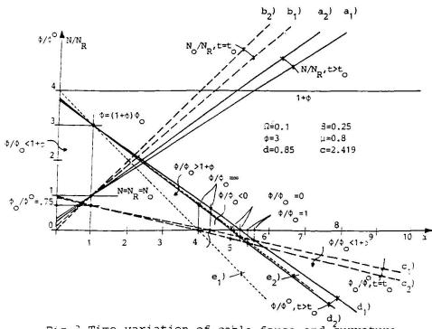
Fig. 2 Time variation of cable force and curvature
