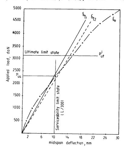
Fig. 3 Load-deflection curves for a test specimen
