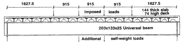
FIG.1.-Arrangement of Test Specimens SF and SP
