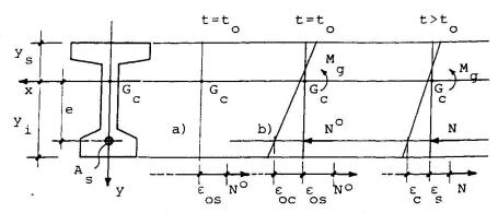
Fig.1 General features of a P.C. section
