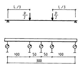
Fig. 2 Typical arrangement for testing slab elements
