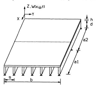
Fig. 1 A typical double-span ribbed plate arrangement
