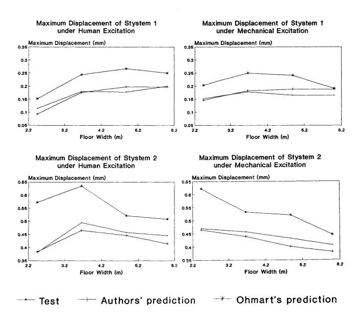
Fig. 2 Predicted vs. test maximum displacement of steel-concrete floors
