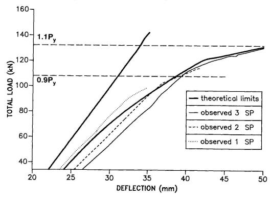
(b) Partial Shear Connection Specimen SP FIG.2.-Observed & Theoretical Load-Deflection Curves for SF & SP
