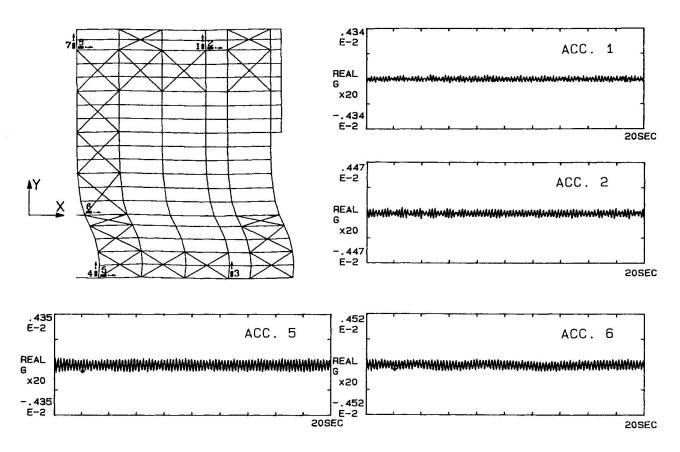
Fig. 4 - Mode 1 of the numerical model (4.39 Hz) and recorded accelerations at 4.5 Hz.
