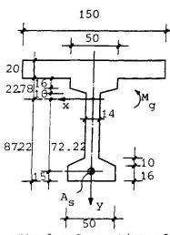
Fig.3 P.C. section of a bridge beam
