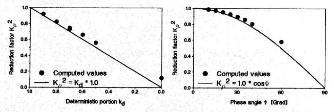
Figure 2: Comparison of the reduction factor with the computed values by means of the power spectral method.
