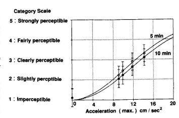
Fig. 6 Vibration acceleration amplitudes and votings
