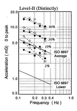
Fig.7 Percentile of Perception to Sinusoidal Motion
