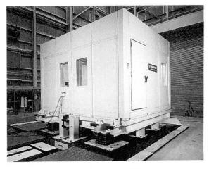
Fig.2 Vibration Simulator
