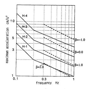
Fig.4. Comparison of perception criteria for wind response
