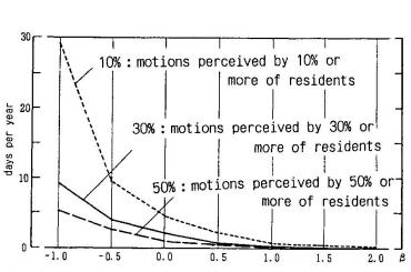
Fig.3. Average number of days for pereption of motions due to wind with  $\beta$
