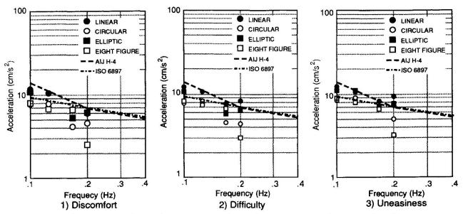
Fig. 7 Relationship between vibration acceleration amplitudes rated 2.5 and existing guidelines
