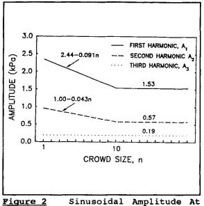
Figure 2 Sinusoidal Amplitude At Dominat Harmonics Vs. Crowd Size
