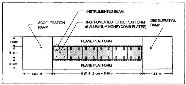
Figure 3 The Force Platform For Measuring Moving Loads
