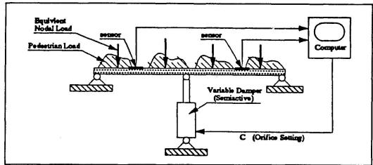
Figure 5 Floor System With Semiactive Damper
