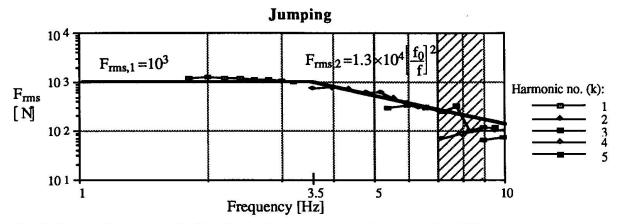
Fig. 8 Narrow-band model of the forces from one person jumping.  $f_0=1$  Hz.
