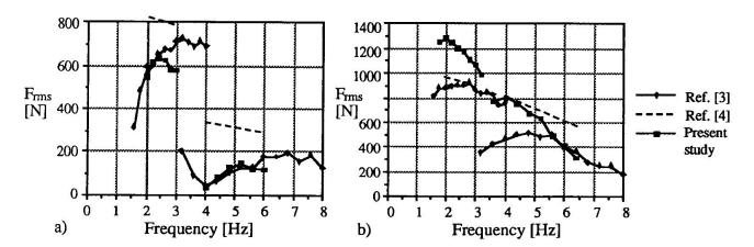
Fig. 5 Comparison of rms force components for the first two harmonics of the forces from a) running and b) jumping.
