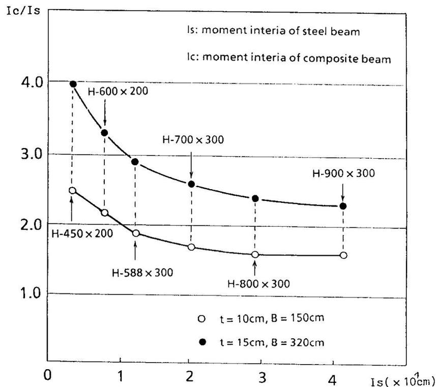
Fig.2 Increase in flexural rigidity of composite beam
