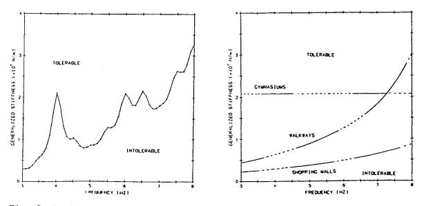
Fig. 5: Design Limits for Reference Walkway Fig. 6: Design Guidelines
