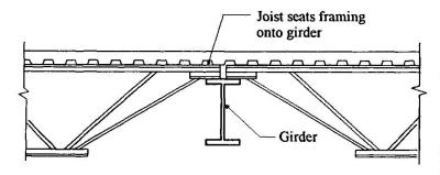
Figure 2 Light Truss Support
