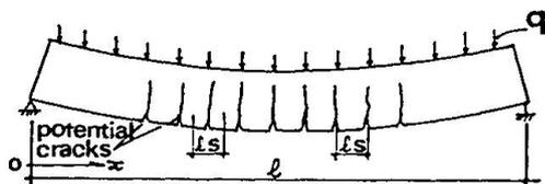
Fig. 1: Model of member with potential cracks.
