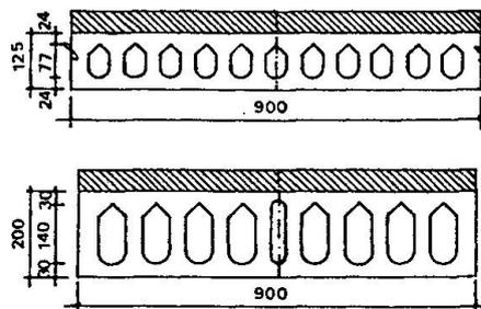
Fig. 2: Sections of analysed floor slabs.
