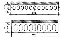
Fig. 2: Sections of analysed floor slabs.
