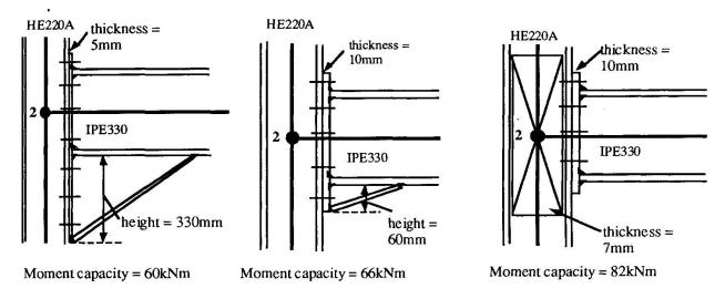
Fig. 7 Functional equivalent connections
