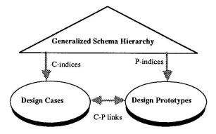
**Figure 1.** The relationships between generalized design schemas, design cases and predefined design prototypes. C-indices means case indices, P-indices means prototype indices, and C-P links means case-prototype links.
