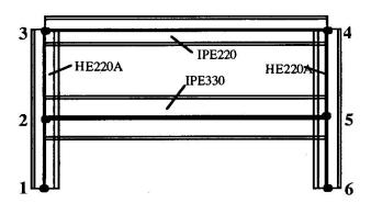
Fig. 5 Portal structure with profiles
