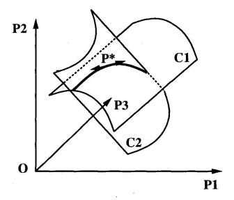
Figure 3: P1/C1, P2/C2 and P3 represent parameters and constraints of three different abstractions. By defining a new parameter,  $P^*$ , which maps to positions on the intersection curve of the two constraints C1 and C2, solutions can be found without unstable iterations through selecting a suitable value for  $P^*$ .
