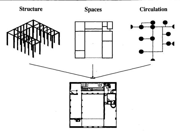
Figure 1: A building represents an integration of many different abstractions, including structure, spaces and circulation pattern.
