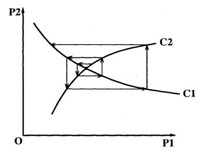
Figure 2: P1/C1 and P2/C2 represent parameters and constraints in two different but interacting abstractions: the correct choice of the parameter is on the constraint curve. When discrepancies in each abstraction are corrected in isolation, the process may diverge as indicated by the arrows.
