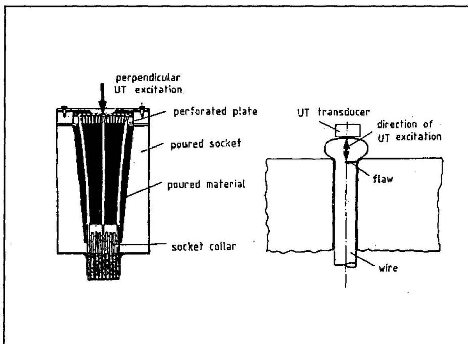
Fig. 3: UT inspection method
