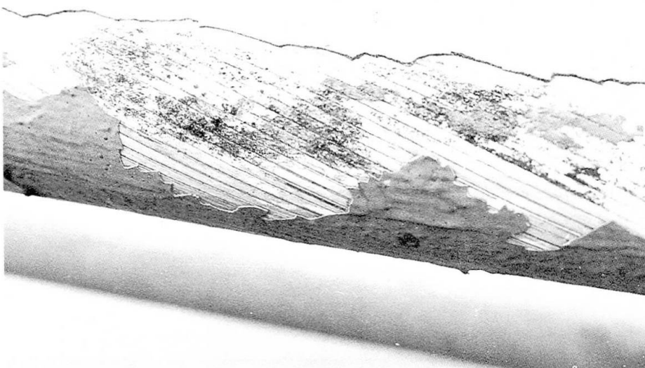
Fig. 11: Corrosion under an undestroyed corrosion protection, detected by EM-inspection
