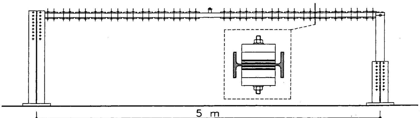
Fig. 8 Steel I beam experimental specimen
