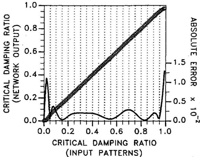
Fig. 5 Rating critical damping ratios in the 0-1 range
