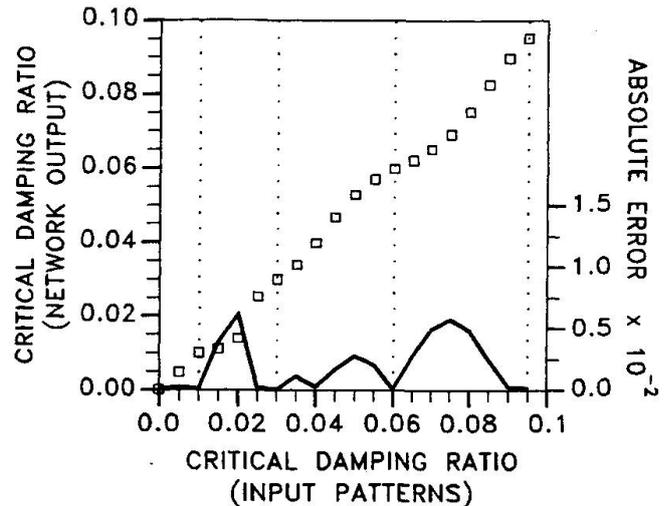
Fig. 6 Rating critical damping ratios in the 0-0.1 range
