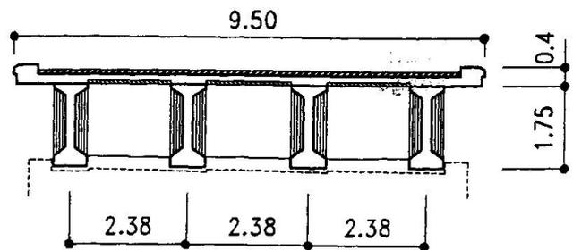
Fig. 9 Bridges cross-section
