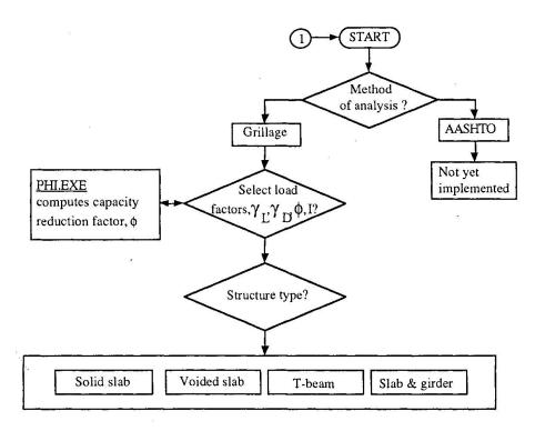
Fig. 1. Load factor selection module
