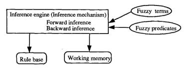
Fig.1 Architecture of Fuzzy Production System
