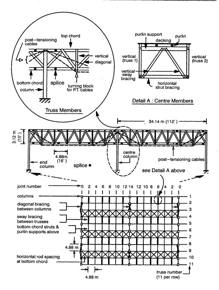
Fig. 1 A double parallel chord Warren truss building
