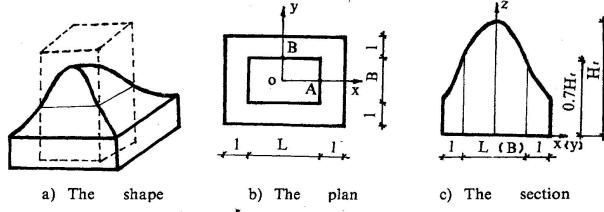
Fig.3 Accumulation model of a overall collapsed building
