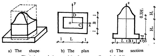
Fig.4 Accumulation model of a top collapsed building
