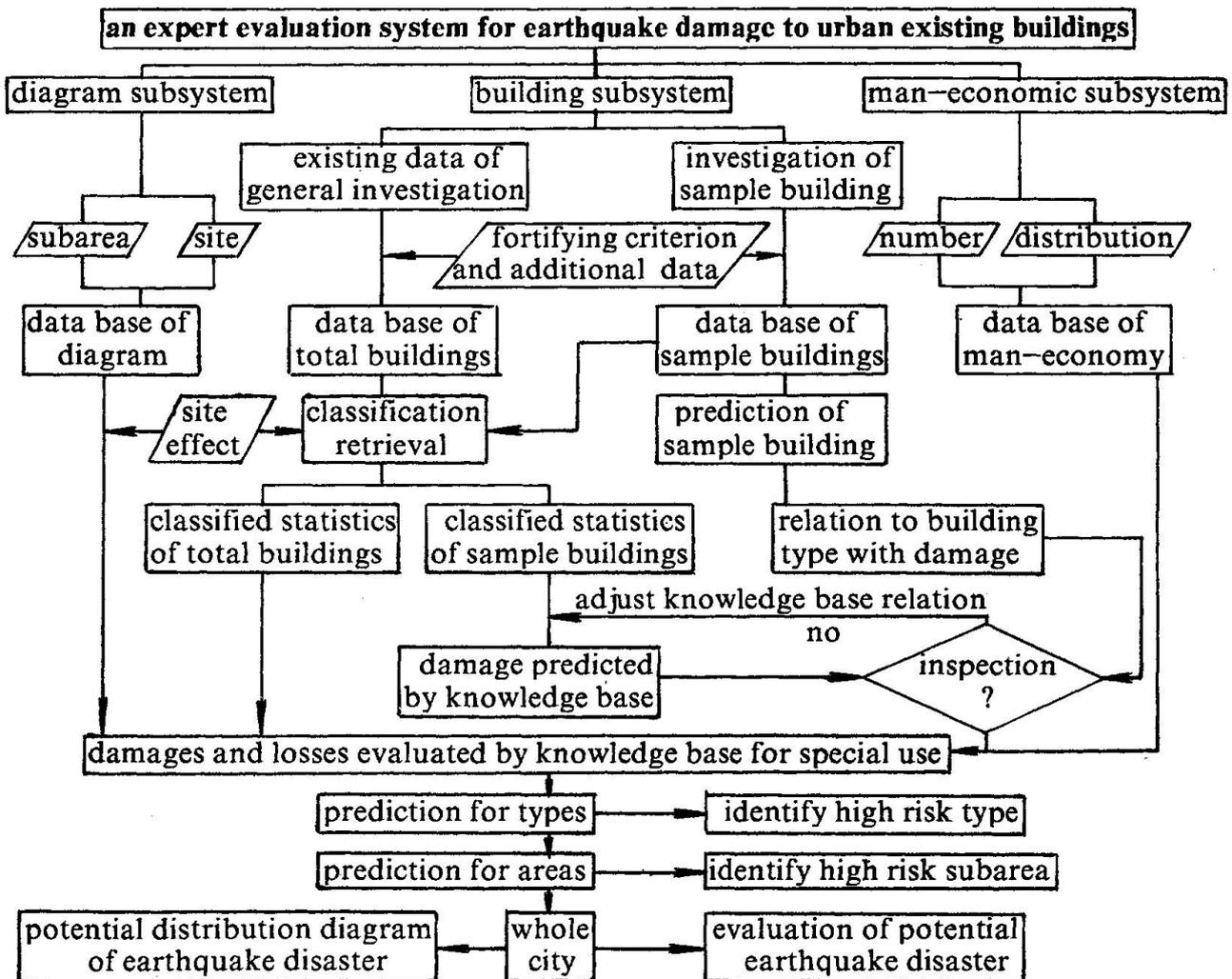
Figure 2. The block diagram of the expert evaluation system PDKSCB-1
