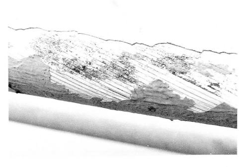
Fig. 11: Corrosion under an undestroyed corrosion protection, detected by EM-inspection
