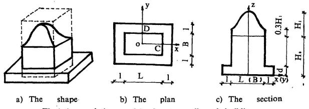
Fig.4 Accumulation model of a top collapsed building
