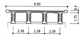
Fig. 9 Bridges cross-section
