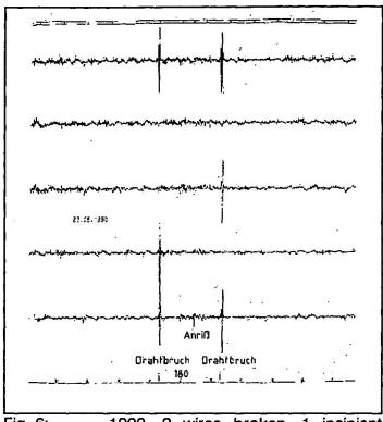
Fig. 6: 1990, 2 wires broken, 1 incipient crack
