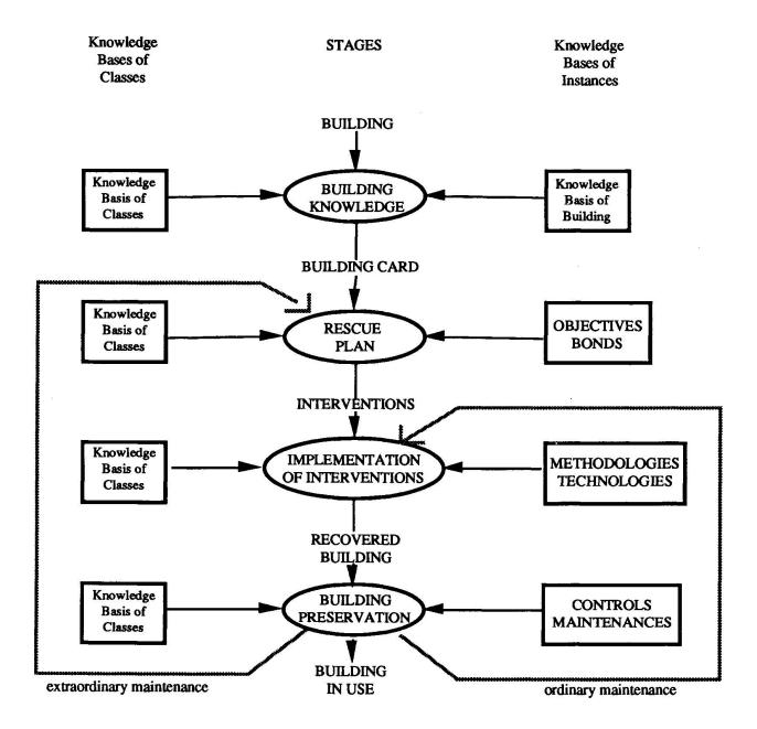
fig. 1 General Model of the SMIRNE System's domain: the model of recovery stages
