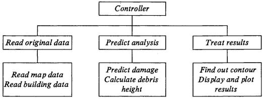
Fig.1 Functional modules diagram of PEDDD
