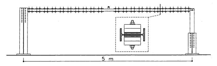
Fig. 8 Steel I beam experimental specimen
