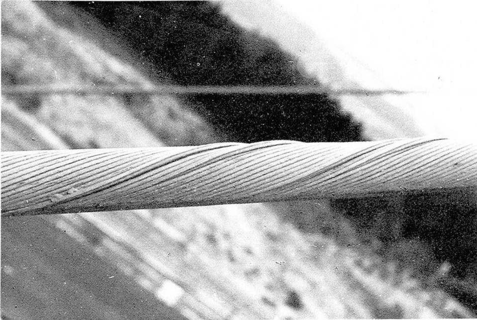
Fig.1: Mechanical distortion
