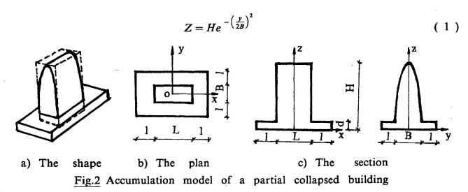
To describe the debris that come from the collapsed wall, the average thickness d in the involved range l is used. Assume that the wall are broken one story by one story, distance l to the horizontal position of the debris of the top story can be determined by Eq.(2).
