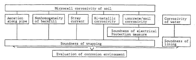
Fig. 2 The conceptual structure of corrosion environment factors
